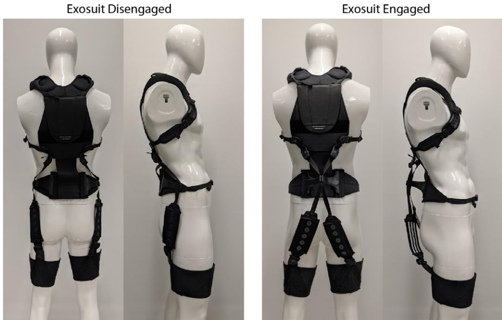
**Figure 2.** Photos of the extensible exosuit prototype in disengaged mode (two photos on the left), and in engaged mode (two photos on the right). Refer to the schematic in Figure 6 for call-outs to each component.
