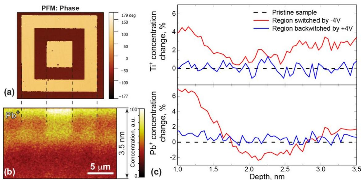
**Figure 1.** Local chemical changes in the bulk of PZT film, induced by local polarization switching. (a) PFM phase of polled regions; (b) corresponding ToF-SIMS X-Z map of  $\text{Pb}^+$  distribution; (c) depth profiles of local concentration changes with respect to the pristine sample of  $\text{Ti}^+$  (*top plot*) and  $\text{Pb}^+$  (*bottom plot*) within outer square switched by negative bias (*red line*) and middle square backswitched by positive bias (*blue line*).
