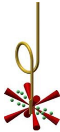
Figure 1. Schematic view of the experimental setup at the Shenguang-II laser facility. Eight laser beams at 351 nm were divided into two bunches and focused onto both sides of the planar plate simultaneously.
