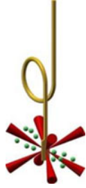
Figure 1. Schematic view of the experimental setup at the Shenguang-II laser facility. Eight laser beams at 351 nm were divided into two bunches and focused onto both sides of the planar plate simultaneously.
