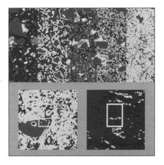
ON THE COVER: The five sections of the upper half of this photo, from left to right, show different stages in a microstructure development model of Portland cement hydration. The first section shows the initial particles before the beginning of hydration. The fifth section shows the cement-to-water mixture after 76% of the cement has hydrated, with the dominant product phase being the yellow calcium silicate hydrate gel surrounding the particles.
