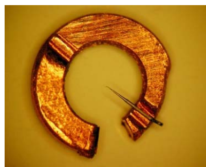
Fig.2. The coupon designed for top-side milling with one tip attached.
