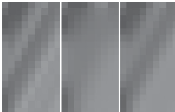
Fig. 5. Left: original intra prediction. Middle: uniformly filtered prediction as in subsection III.A. Right: signal adaptive filtered prediction as in subsection III.B.
