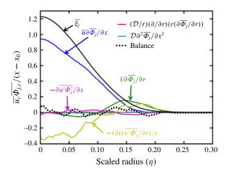
FIGURE 9. (Colour online) The budget of (3.10) versus the scaled radius. Budget terms are normalised by  $\overline{u_c}\overline{\Phi_{j,c}}/(x-x_0)$  and averaged over normalised axial distances x/D = 15-40.
