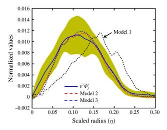
FIGURE 10. (Colour online) Comparison of the models proposed in (3.11), (3.12) and (3.15) with the DNS data of normalised radial flux of mass-weighted stream age,  $\overline{v'\Phi_j'}/\overline{u_c}\overline{\Phi_{j,c}}$  (shaded area), plotted against the scaled radius,  $\eta$ . Fitting parameters are  $\beta_1 = 0.0015$ ,  $\beta_2 = 0.016$  and  $\beta_3 = 0.01$ .
