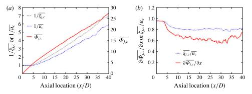
FIGURE 7. (Colour online) Axial variation of: (a) the centreline average of mass-weighted stream age  $\overline{\Phi_{j,c}}$  (right axis) and the reciprocals of the centreline average mixture fraction  $1/\overline{\xi_{j,c}}$  and axial velocity  $1/\overline{u_c}$  (left axis); (b) the axial gradient of  $\overline{\Phi_{j,c}}$  and the ratio of  $\overline{\xi_{j,c}}$  and  $\overline{u_c}$  along the centreline.
