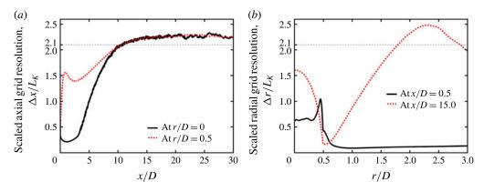
FIGURE 1. (Colour online) The ratios between the grid spacing and the calculated Kolmogorov length scale along (a) the axial direction and (b) the radial direction.
