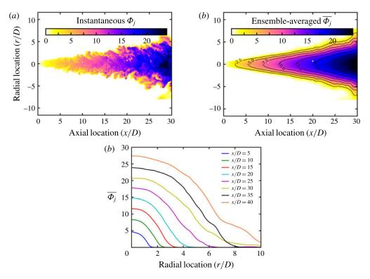
FIGURE 6. (Colour online) (a) Instantaneous mass-weighted stream age,  $\Phi_j$ , (b) ensembleaveraged  $\overline{\Phi_j}$  fields on a section through the jet centreline and (c) the radial variation of  $\overline{\Phi_j}$  at different axial locations.
