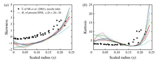
FIGURE 12. (Colour online) (a) The skewness and (b) the kurtosis of mass-weighted stream age over the scaled radius.
