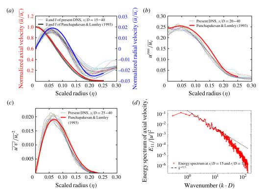
FIGURE 2. (Colour online) Radial profiles of (a) the mean axial velocity, (b) the axial velocity fluctuation, (c) the axial-radial Reynolds stress and (d) the energy spectrum of axial velocity.
