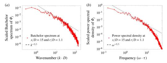
FIGURE 13. (Colour online) (a) Energy spectrum of mass-weighted stream age and (b) power spectrum by direct Fourier transform of the mass-weighted stream age at x/D = 15 and r/D = 1.1.
