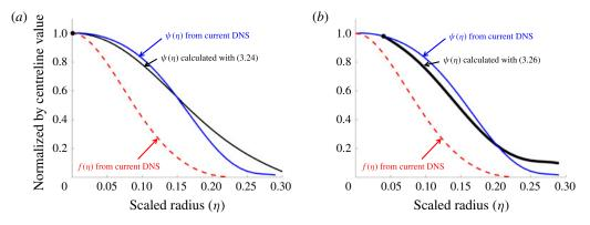
FIGURE 11. (Colour online) Comparison of the mass-weighted stream-age shape function profiles over the scaled radius between the current DNS data and solutions from (a) (3.24) and (b) (3.26). The parameters used are  $\beta_1 = 0.0038$ ,  $\beta_3 = 0.01$  and  $B/(A\alpha) = 1.33$ .
