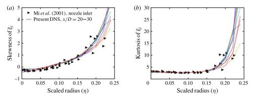
FIGURE 4. (Colour online) The skewness (a) and the kurtosis (b) of the mass fraction over the scaled radius at different axial locations.
