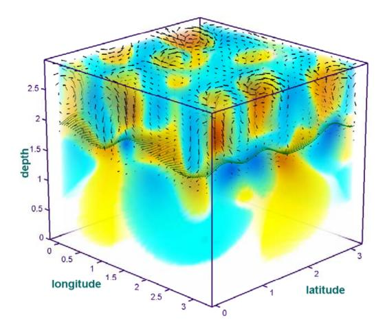
Figure 1. Distribution of temperature disturbances and velocity field in the layer with deformable interface
