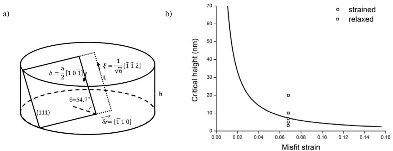
**Figure 3.** (a) The simplified model of a QDs with a dislocation loop expanding across the QD. (b) The critical height of QDs to form dislocation loops vs the misfit strain between dots and matrices. Experimental data are also shown in the graph.
