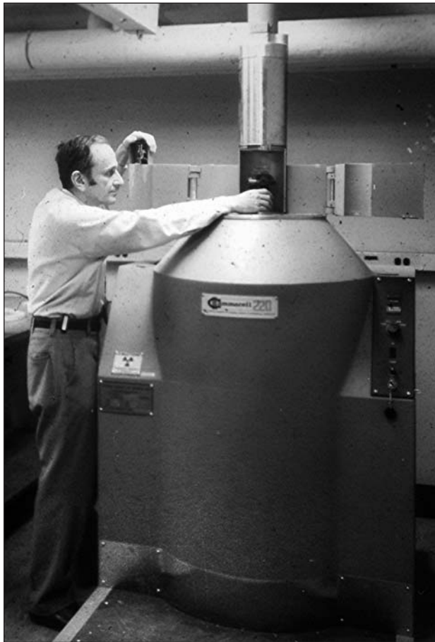
Kurt Nassau, at Bell Labs, conducting an irradiation experiment in a Cobalt-60 gamma cell.
