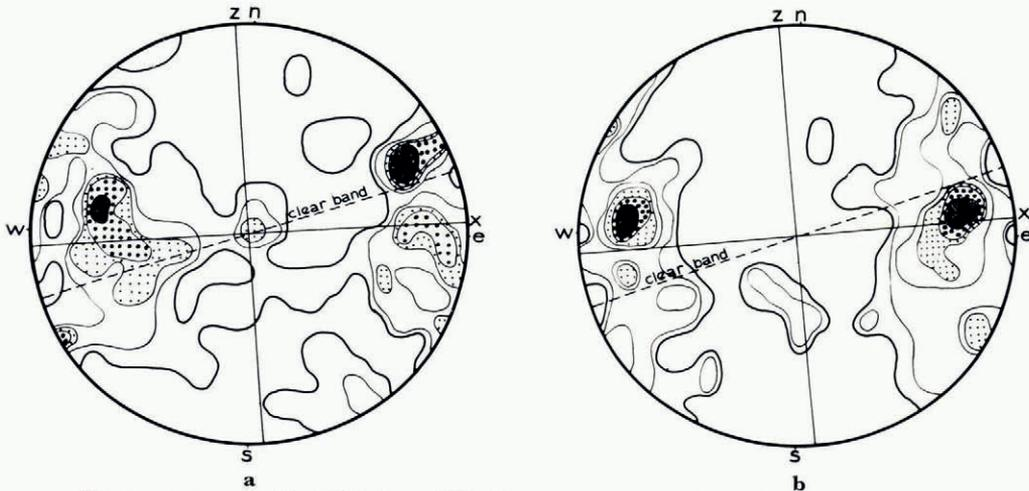
Fig. 5. a. 224  $c$ -axes of ice (CF2) from grid F. Contours 1-2-3-4-5  $<$ %; maximum 5% per 1% area. Grain-size: 1.1 grains/cm<sup>2</sup>.
