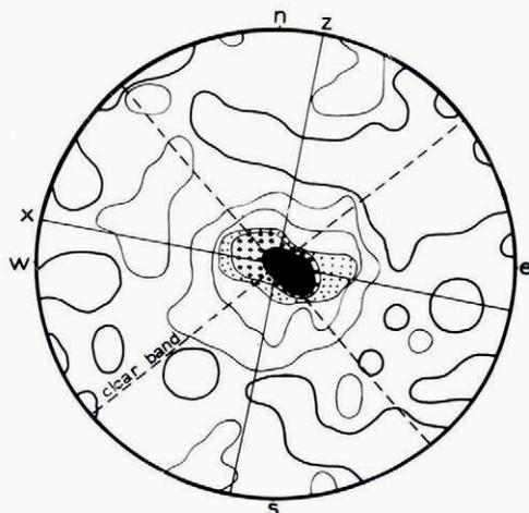
Fig. 3. 330  $c$ -axes of ice (CH1) from grid H.\* Contours 1-2-3-4-5-6 < %; maximum 7% per 1% area. Grain-size: 19 grains/cm<sup>2</sup>.
