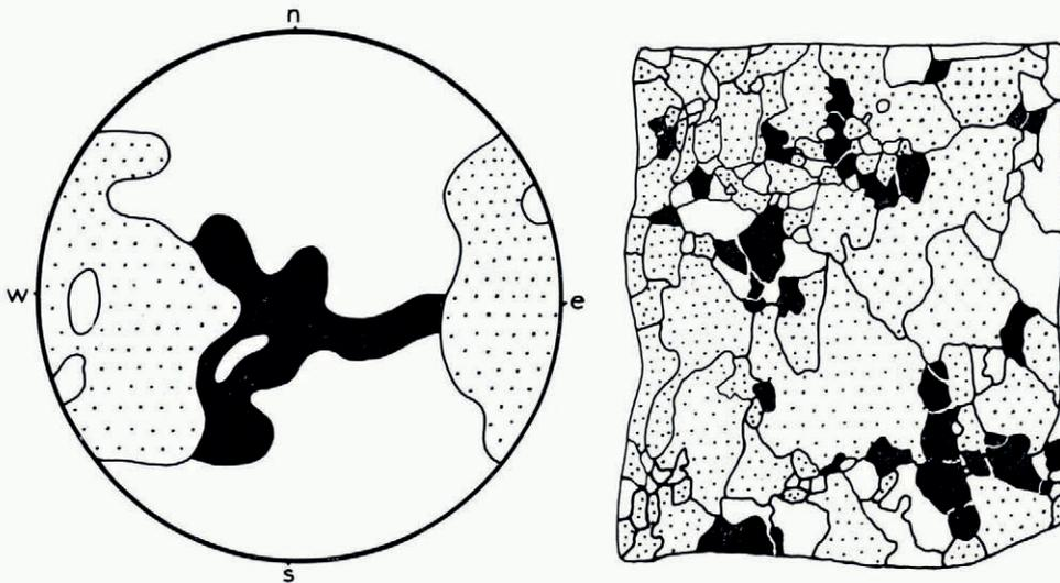
Fig. 6. Axis-distribution diagram of CF2. Thin section of the ice is  $12 \times 10$  cm.
