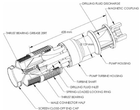
Fig. 4. Pump section.
