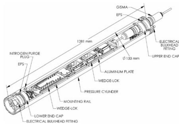
Fig. 5. Instrument section.
