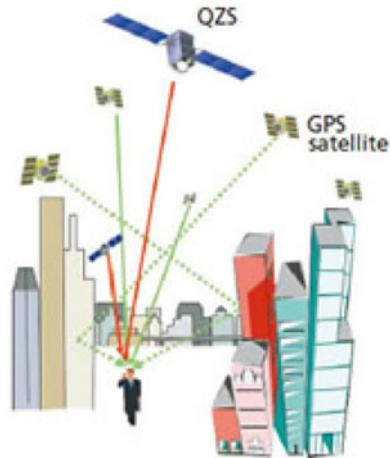
Figure 1. Assistance of QZSS for GPS positioning in high-rise urban areas (Courtesy of JAXA).
