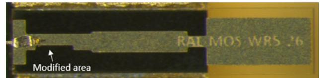
**Fig. 6.** Revised WG-MS transition in all 183 GHz LNAs for MetOp-SG. The modified cut is highlighted. The coplanar output line on the MMIC is to the left of the transition. The waveguide channel is to the right of the transition.
