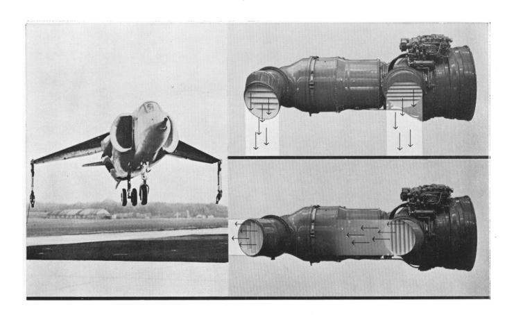
The new Bristol Siddeley BS 53 high-ratio turbofan represents a major engineering breakthrough in the field of aircraft propulsion.
