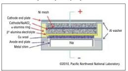
design also incorporates a thin layer of solid electrolyte, which also lowers the resistance. Because of the decrease in resistance, the battery can af-
