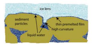
**Fig. 2.** Geometry of the ice—liquid interface near the base of an ice lens. Separate regions are highlighted in which liquid water forms a thin premelted film that separates the ice from the sediment particles where their surfaces are in close proximity and the area of high surface curvature where the ice—liquid interface is comparatively distant from the sediment particles.
