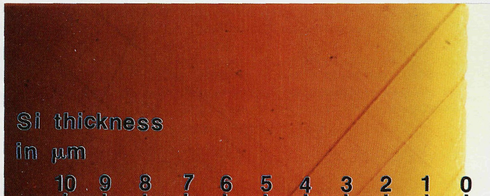
Figure 2: The colors of a thin, backlit wedge of single-crystal silicon. The dark, diagonal lines are cracks along silicon (111) crystal planes. The lighter lines and spots are polishing scratches and dust particles, respectively
