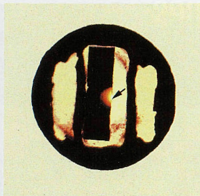
Figure 1: Cross-sectional TEM sample of indium tin oxide (ITO) on glass, prepared with an adjacent piece of silicon used as a thickness indicator
