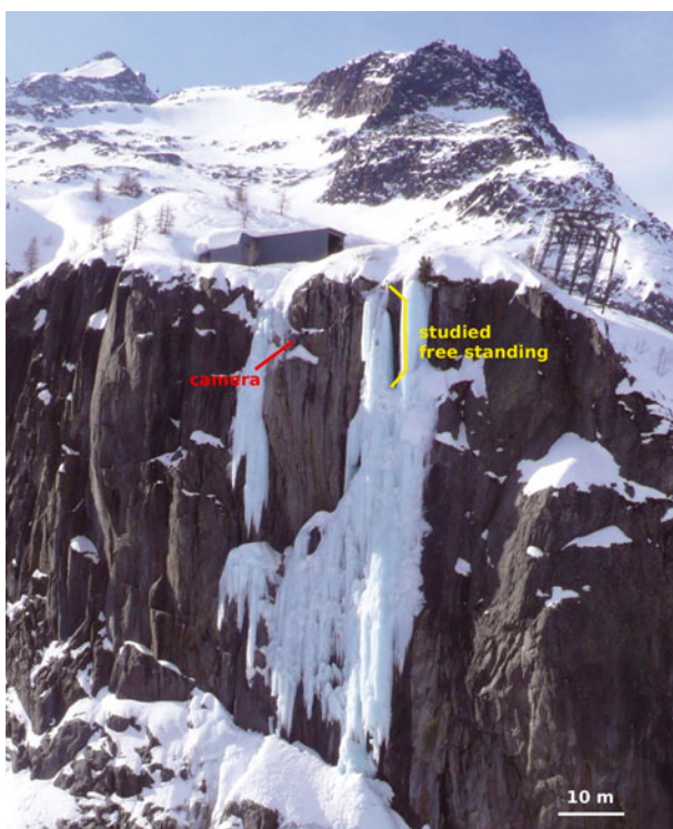
Fig. 2. Overall view of the Nuit Blanche frozen waterfall. Cameras view the top free-standing section, where sampling and pressure measurements were performed.
