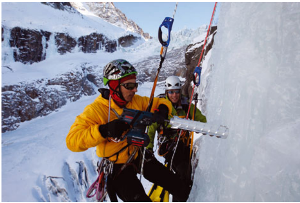
Fig. 5. Coring in the Nuit Blanche free-standing section.
