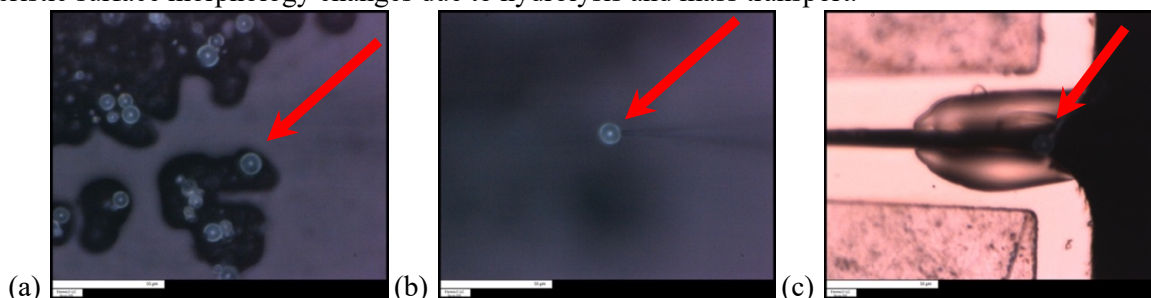
Figure 2. (a) particle identification, (b) particle removal via micromanipulation, (c) particle manipulated to glue on EXpressLO™ slotted grid.
