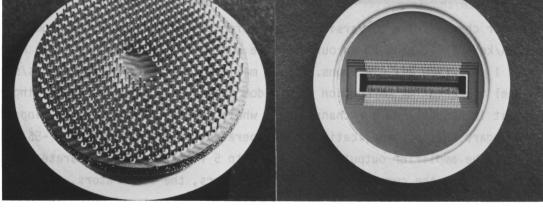
Fig.4 Ceramic header: backside and frontside with mounted array
