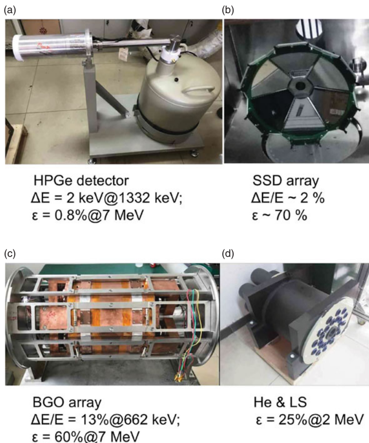
Figure 4. The HPGe, BGO, neutron and charged particle detector arrays for JUNA.
