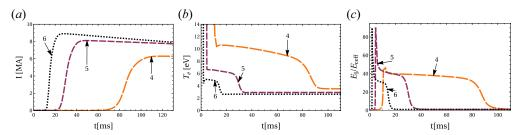
FIGURE 4. Time evolution of quantities of interest for the low  $n_{D,\text{inj}}$  representative cases: C4–C6. Line colour darkens and dashes shorten with increasing case number, and case numbers are indicated with callouts. (a) Runaway electron current. (b) Electron temperature at mid-radius. (c) Electric field normalized to critical electric field at mid-radius. (Note the longer time range plotted in panel a.)
