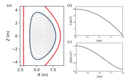
FIGURE 8. (a) Magnetic geometry with flux surfaces (grey curves), the outermost modelled flux surface r=a is indicated by the thick blue line, and the effective wall is shown in red. The rest of the panels show initial plasma parameter profiles. (b) Electron temperature. (c) Current density.
