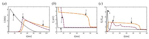
FIGURE 3. Time evolution of quantities of interest for the high  $n_{D,\rm inj}$  representative cases: C1–C3. Line colour darkens and dashes shorten with increasing case number, and case numbers are indicated with callouts. (a) Runaway electron current. (b) Electron temperature at mid-radius. (c) Electric field normalized to critical electric field at mid-radius. (Note the longer time range plotted in panel a.)
