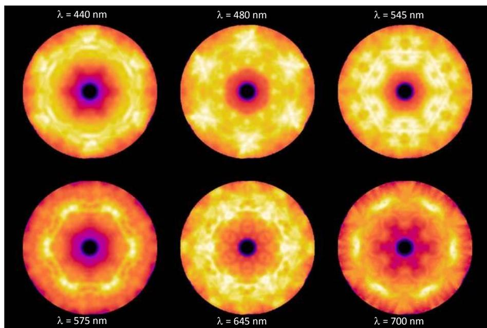
**Figure 3.** Wavelength-filtered emission patterns (normalized by intensity) extracted from the wavelength- and angle-resolved cathodoluminescence data cube (670 emission patterns in total), central wavelength as indicated, bandpass  $\pm 1.5$  nm. Angular scale annotations removed for clarity but are identical to that displayed in Figure 2.
