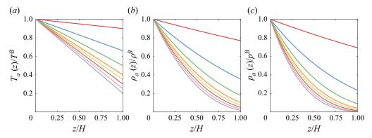
Figure 1. Adiabatic equilibrium profiles of the thermodynamic state variables. (a) Temperature T, (b) density  $\rho$  and (c) pressure p. The difference between top and bottom values for all three variables increases with D, see table 1 for the colour code description.
