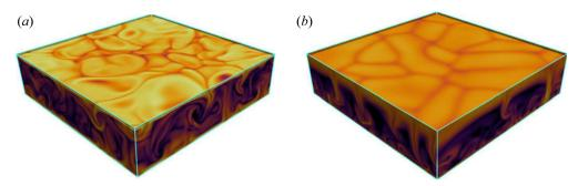
Figure 2. Visualization of the plume structure of the superadiabatic temperature field  $T_{sa}$ . Contours of  $\ln |\nabla T_{sa}|$  are shown at two instants, (a) for case 1 with D=0.1 and (b) for case 8 with D=0.8. Minimum/maximum contour levels correspond to -7.0/-2.4 in (a) and -9.5/-4.0 in (b). The top contour surface is slightly below z=H.
