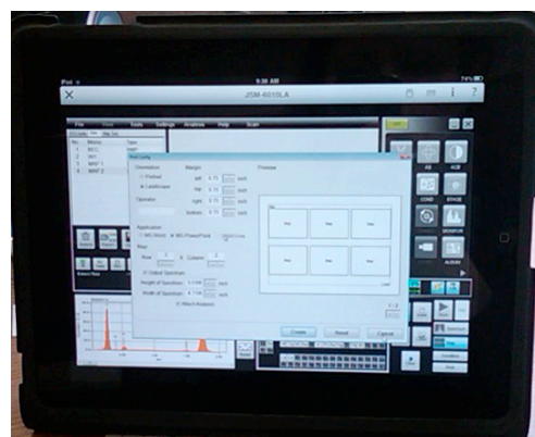
Figure 2. Example of the VNC interface connected to an FEG-SEM (left), and InTouch Scope EDS interface (right) on an Apple iPad.
