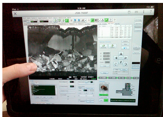
Figure 2. Example of the VNC interface connected to an FEG-SEM (left), and InTouch Scope EDS interface (right) on an Apple iPad.
