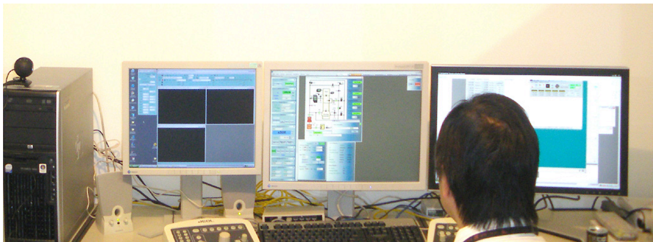
Figure 1. Remote operation of the JEM-ARM200F. The remote station uses the same GUI and hardware interface as local operation of the microscope.
