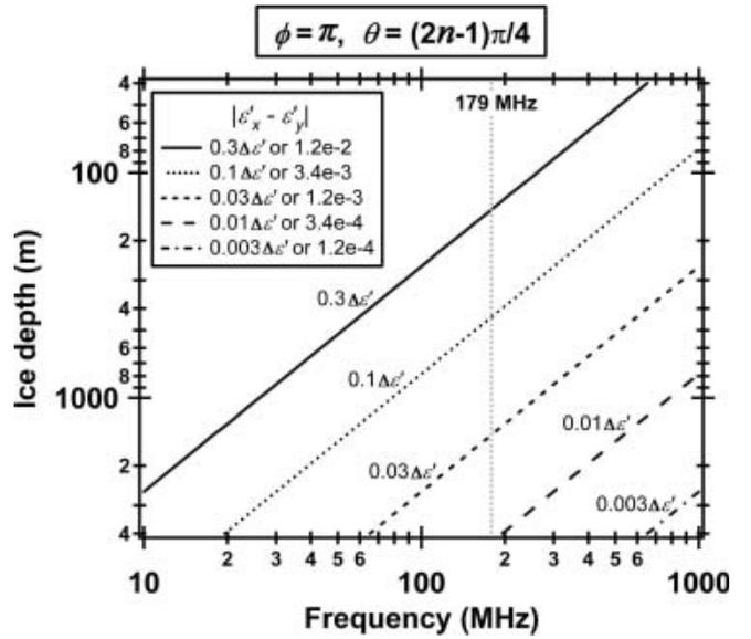
**Fig. 6.** Depths at which the shallowest co-polarized node ( $\phi = \pi$ ) occurs are shown in terms of the radar frequency and the COF dielectric anisotropy.  $\Delta\varepsilon'$  is the dielectric anisotropy of pure-ice single crystals. The vertical line at 179 MHz indicates the radar frequency used in our simulations and in observations.
