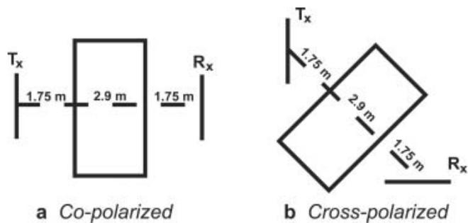
**Fig. 2.** Top views of antenna arrangements for (a) co-polarization and (b) cross-polarization measurements. For both arrangements, the transmitting ( $T_x$ ) and receiving ( $R_x$ ) antennae are at opposite sides of the snow vehicle (shown as a rectangle). The centers of the three-element Yagi antennae are 3.2 m above the ice-sheet surface.
