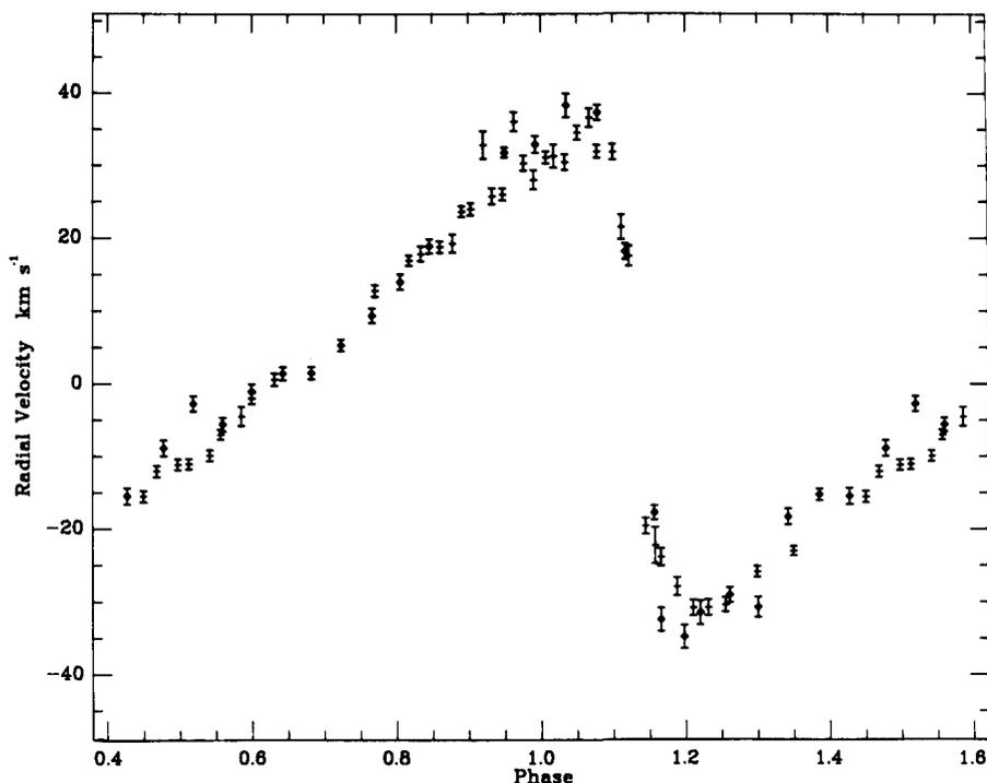
Figure 1. The radial velocity curve of V652 Her obtained with the AAT in 1982. Exposures were for 300 s at 10 Å/mm with the IPCS on July 2 (horizontal bars) and for 200 s at 26 Å/mm with a CCD on July 3 (diamonds).
