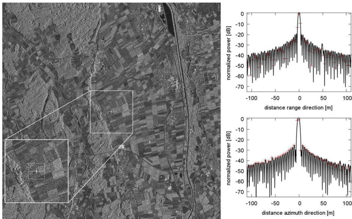
**Fig. 2.** Sentinel-1A SAR image (left) of a scene containing the impulse response of a DLR transponder (center). The area around the point target is zoomed out within the white square at the bottom left corner. The pixel power, related to the target impulse response (right), is extracted from the SAR image along a cut in range (horizontal) and azimuth (vertical) dimension. The black lines depict the interpolated response based on used SAR image pixels (red crosses).
