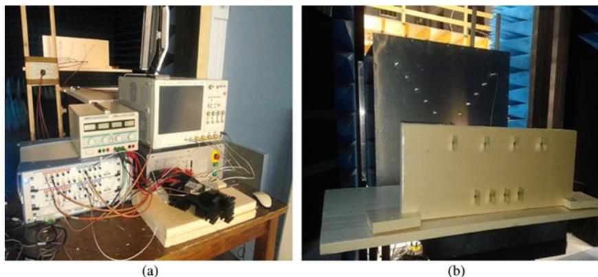
Fig. 5. MIMO Radar measurement setup. (a) Conventional MIMO with four FH-waveforms generated by an arbitrary waveform generator (AWG). (b) Mode-mixing MIMO measurement setup, the transmitters are connected to the metallic cavity behind and the receivers are connected to a digital oscilloscope.
