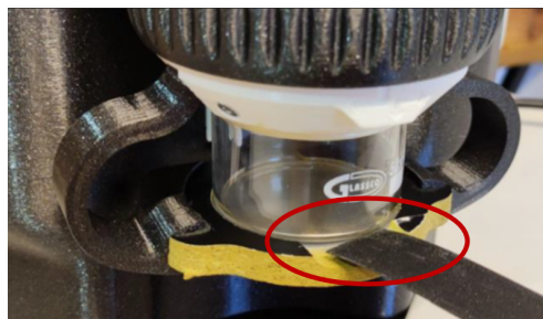
Figure 11. Final redesign of the compliant arms without gap between heating plate and glass.
