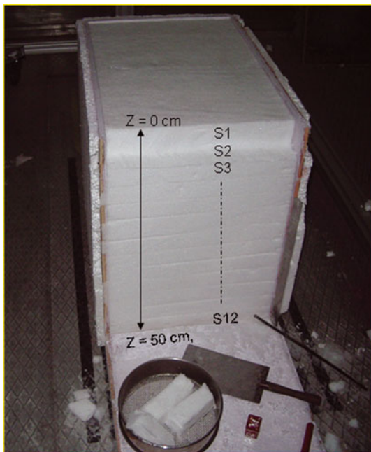
Fig. 2. Sub-layer stratification within a homogeneous block of snow of small rounded grains (class 3a).
