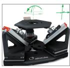
attocube has developed the six degrees of freedom hexaCUBE positioning system. The hexaCUBE combines extremely stiff design and long travel range with nanometer repeatability in 6D. The hexaCUBE combines six (linear) closed-loop piezoelectric motors within an assembly of highest precision ball joints and linear bearings, enabling true motion in 6D
