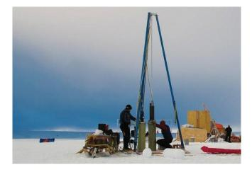
**Fig. 6.** The BID coring at the surface on Taylor Glacier. Notice the anti-torque handles attached to the outer barrel via a clamping device for near-surface coring. Photo by Robb Kulin.
