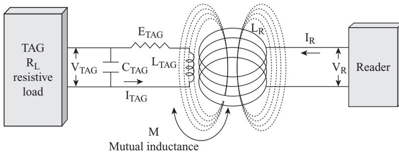
**Figure 2.3** Resonant frequency in tags with inductive coupling.
