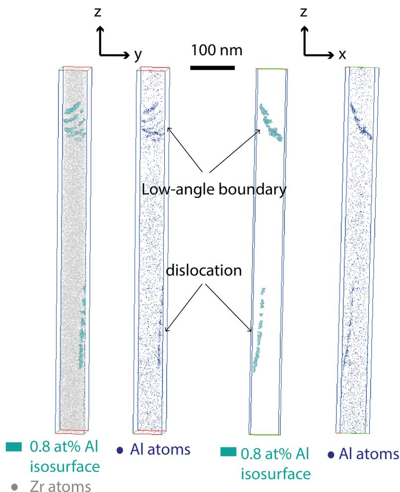
**Figure 1.** Atom probe tomography (APT) reconstructed volume of a distorted Zircon with a sub-grain boundary decorated with Aluminium with a 0.5 at.% Al iso-concentration map. The dataset is shown from two different angles, so that the low angle boundary can be distinguished from the dislocation.
