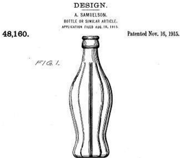
Figure 2.1 Bottle or similar article, US Patent No. D48,160 (Nov. 16, 1915). The design won a national competition sponsored by the Coca-Cola Company to create a new bottle shape for its product.
