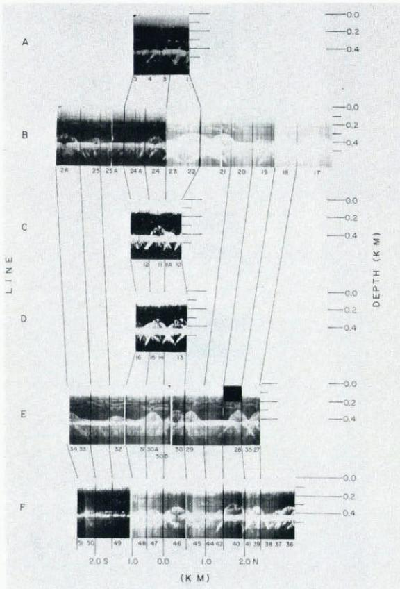
Fig. 3. North-west-south-east data collected with antennae parallel. The numbers are used to identify reflection hyperbolae and are positioned approximately below the vertex. The dark lines between profiles connect corresponding flagged positions on each profile. Profile lengths vary due to different sweep and vehicle speeds.
