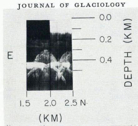
Fig. 9. Crevasse 28 showing two hyperbolae generated at the base of the crevasse (depth 0.42 km) and separated by about 130 m. The vertices are positioned horizontally at about  $1.9^\circ$  N. and  $2.0^\circ$  N., respectively.
