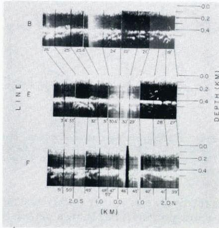
Fig. 5. North-west–south-east data collected with antennae collinear. The numbers are used to identify features and, except for 52', correspond to the numbers in Figure 3. Primes are used to differentiate a feature observed on the collinear data from the same feature on the parallel data. The dark lines between profiles connect corresponding flagged positions on each profile. Profile lengths vary due to different sweep and vehicle speeds.
