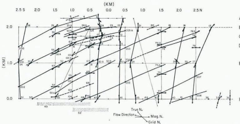
Fig. 6. Crevasse map with identifying numbers corresponding to those on Figures 3, 4, and 5. The heavy solid lines represent crevasses. Dashed lines indicate possible crevasse locations, although the evidence may be weak. The stippled bands at the bottom of the map represent poorly-defined features that may run parallel to the F line. Their position below the F line is arbitrary. The arrows are strike directions calculated from the shapes of the reflection hyperbolae.
