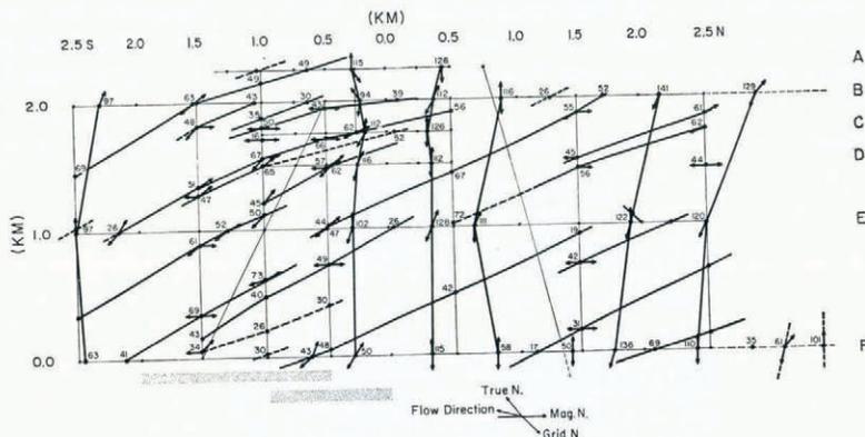
Fig. 7. Crevasse map showing crevasse heights. The heavy solid lines represent crevasses. Dashed lines indicate possible crevasse locations although the evidence may be weak. The stippled bands at the bottom of the map represent poorly defined features that may run parallel to the F line. Their position below the F line is arbitrary. The arrows are strike directions calculated from the shapes of the reflection hyperbolae.
