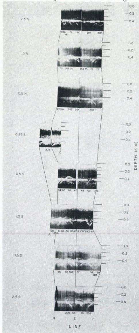
Fig. 4. North-east–south-west data collected with antennae parallel. The numbers are used to identify features and are positioned approximately below the vertex. The dark lines between profiles connect corresponding flagged positions on each profile. Profile lengths vary due to different sweep and vehicle speeds.
