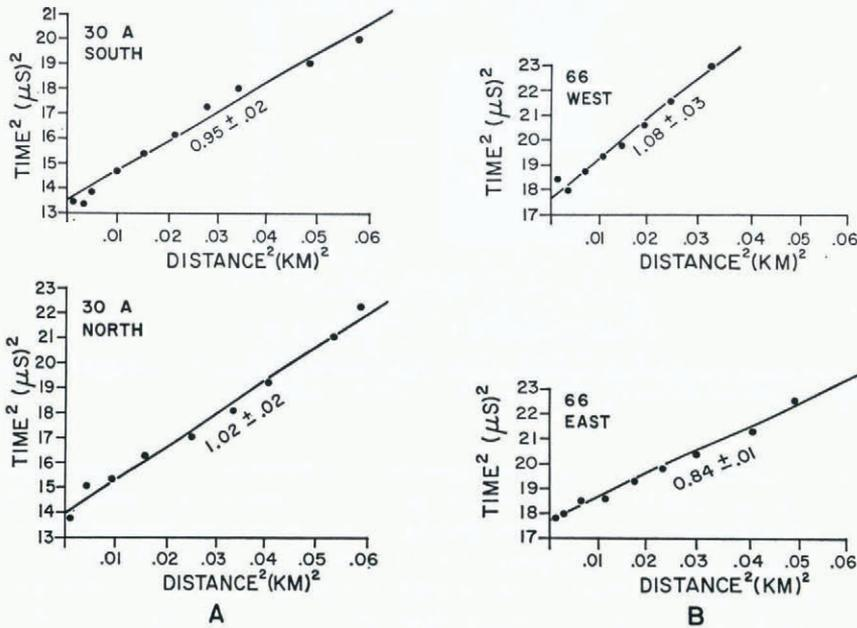
Fig. 8.  $T^2$  against  $x^2$  plots from which strike arrows are calculated. The number below the line fit to each set of data is the calculated value for  $\sin \theta$ . Reasons why this value may be greater than one are discussed in the text. A shows a sample crevasse from set I, B a sample crevasse from set II.
