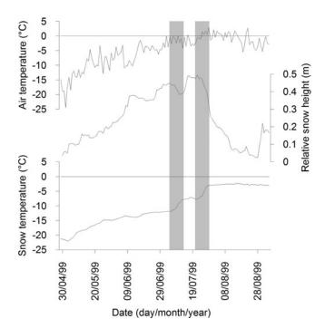
**Fig. 2.** Data from an AWS near the drilling site for time period May–August 1999: air temperature (2.5 m above snow cover at the start in May 1999), relative snow height (relative to start in May 1999) and snow temperature (0.5 m below snow cover at start in May 1999). The horizontal black lines indicate 0°C. Grey shaded areas indicate infiltration events with decreasing snow height and increasing snow temperature.
