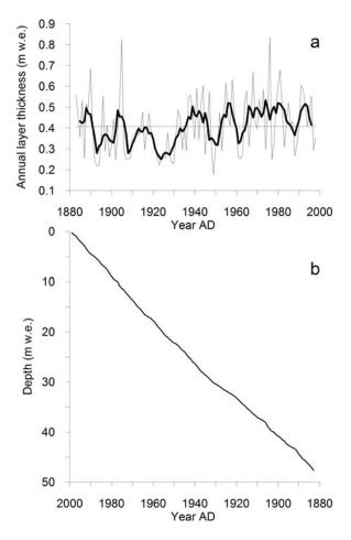
**Fig. 3.** (a) Thickness of the thinned (not decompressed) annual layers (grey line: annual values; thick black line: 5 year running mean (5yrm) values; horizontal line: long-term mean) and (b) depth–age relationship as result of the age model.
