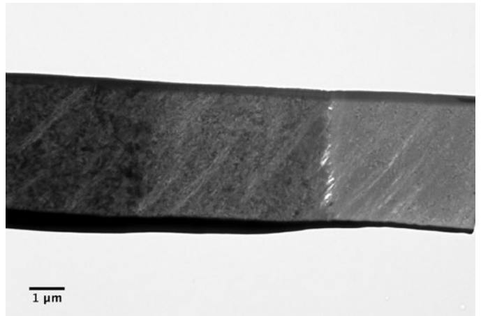
Figure 4: Bright field image of a FIB processed section of a chiton tooth showing the magnetite region (left), goethite/lepidocrocite region (right), and calcium apatite region (right). The dark layer at the bottom of the section is the Pt protective layer deposited during the FIB processing.
