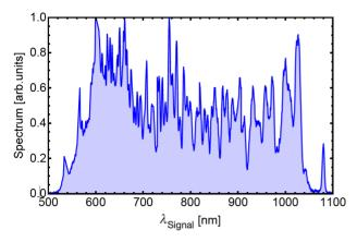
Figure 6. Noncollinear OPA stage seed: supercontinuum generation.
