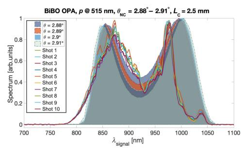
Figure 8. Experimental results for the BiBO NOPA stage: amplified spectrum for a 2.5 mm crystal. Different noncollinear angles are plotted to show the influence of  $\theta_{NC}$  on the spectral dip around 920 nm.
