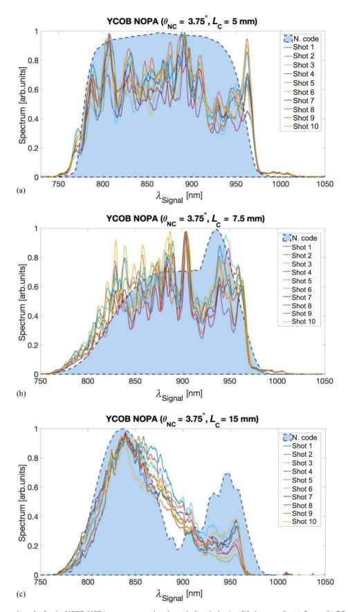
**Figure 7.** Experimental results for the YCOB NOPA stage compared to theoretical analysis. Amplified spectra for (a) 5 mm, (b) 7.5 mm and (c) 15 mm crystals. The shadowed curve is the numerically calculated amplified spectrum for the following parameters:  $\lambda_p = 515$  nm,  $I_p \sim 50$  GW/cm<sup>2</sup>,  $d_{eff} = 5$ , 7.5, 15 mm YCOB crystal thicknesses, and the signal and crystal angles are those reported in Table 2.
