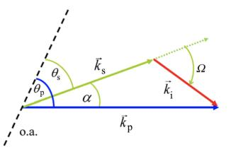
Figure 1. Representation of noncollinear phase-matching condition. o.a. is the crystal optic axis.
