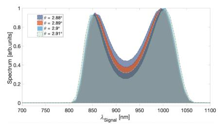
Figure 4. Simulated noncollinear angular dependence of the BiBO amplified spectrum. Crystal thickness is 2.5 mm and the pump intensity is ~50 GW/cm<sup>2</sup>.
