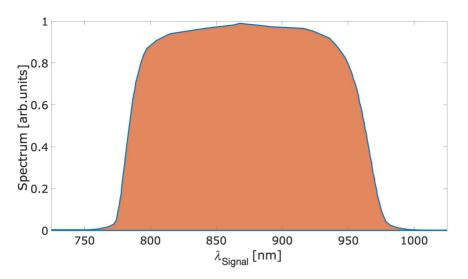
Figure 3. Simulated amplification spectrum for a 5 mm YCOB crystal pumped at 515 nm with an intensity of ~50 GW/cm<sup>2</sup>.
