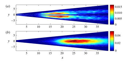
FIGURE 7. Contour maps of (a)  $100\tilde{u}_{rms}^2$  and (b)  $100\tilde{v}_{rms}^2$  for the excited jet at f = 50 Hz.
