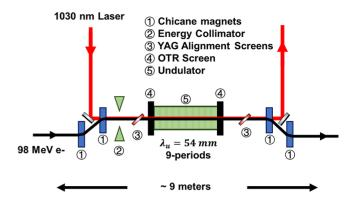
**Figure 2.** The configuration of the LCLS-II laser-heater system, which includes a 1030 nm laser, chicane magnets, optical transition radiation (OTR) screen, energy collimator, pop-in YAG alignment screens (to align the laser and the electron beam) and undulators<sup>[48,49]</sup>.
