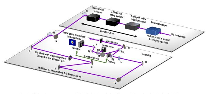
Figure 6. The laser beam transport system for the LCLS-II. Inset: the laser beam profile is monitored by the virtual cathode camera.
