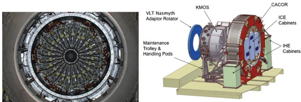
**Figure 1.** The left hand image shows the 24 pickoff arms of KMOS in their retracted positions. The right hand schematic illustrates the position of KMOS on the Nasmyth platform of the VLT.
