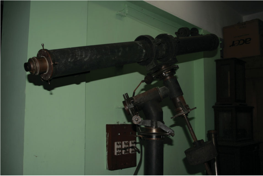
Figure 3. The 95 mm Secrétan telescope.
