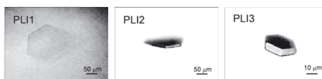
Fig. 1. Typical PLIs observed in the EPICA-DML ice core. All PLIs shown here are from the 1474 m depth sample. PLI1 is the thinnest ( \sim 1\text{--}2\ \mu\text{m} thick), while PLI2 and PLI3 are no thicker than 5\ \mu\text{m} .
