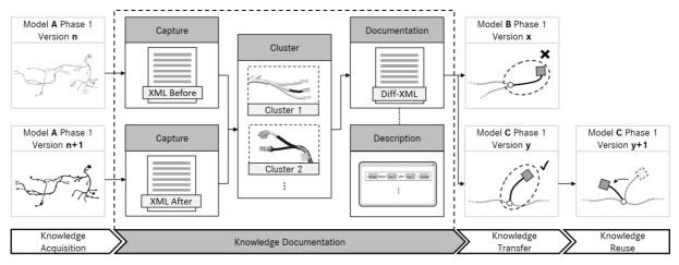
Figure 1. KMS for wiring harness development on the basis of (Eder et al., 2022)
