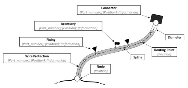
Figure 3. Structure and elements of a wiring harness
