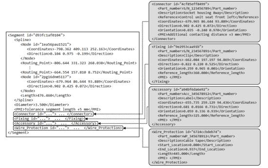
Figure 4. Knowledge representation of a wiring harness segment in XML scheme
