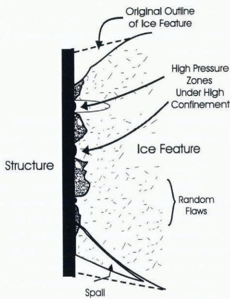
Fig. 1. Schematic of high-pressure zone.
