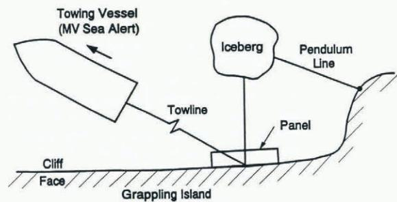
Fig. 2. Schematic of iceberg-impact test configuration (plan view).
