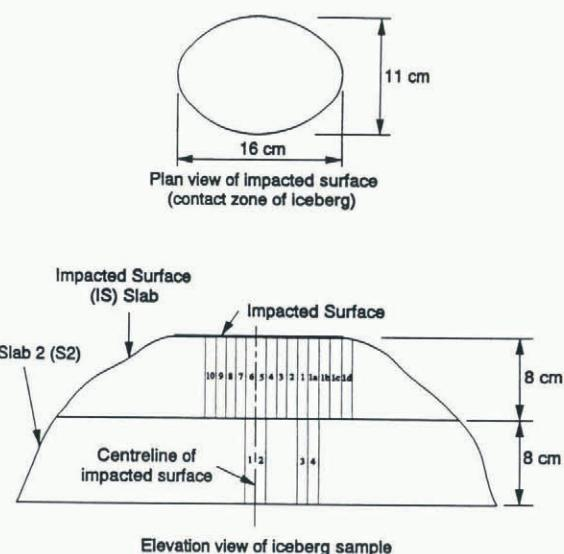
Fig. 3. Schematic of iceberg sample containing contact zone and position of thin sections.
