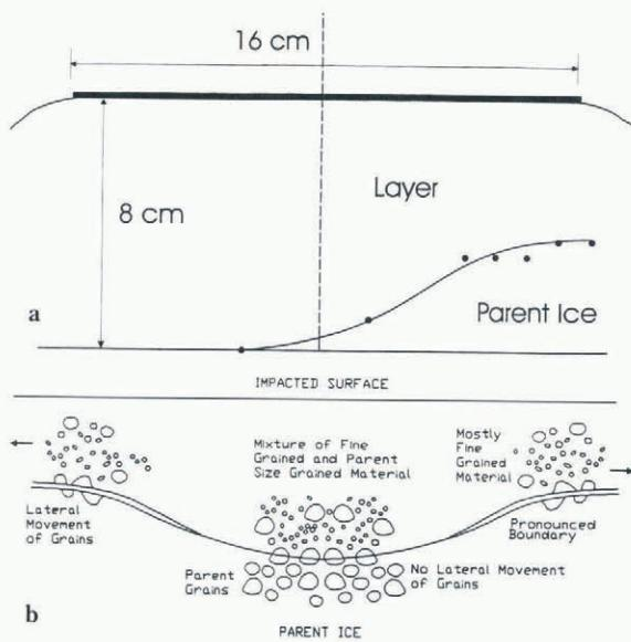
Fig. 4. Schematic drawings of profile of layer with most microstructural change. (a) Schematic of profile based on measurements of layer depth in thin sections. (b) Sketch of profile shape of the contact zone.
