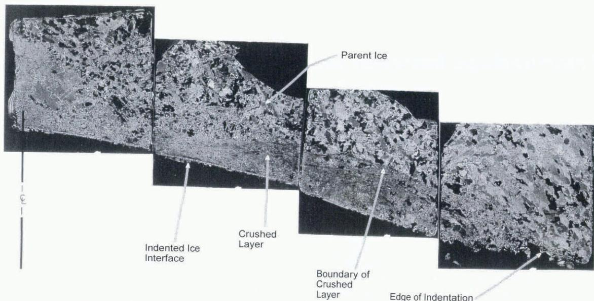
Fig. 5. Section across crushed layer after spherical-head indentation test, Hobson's Choice ice island, 1989 (photo taken by E. Stander and used with permission).
