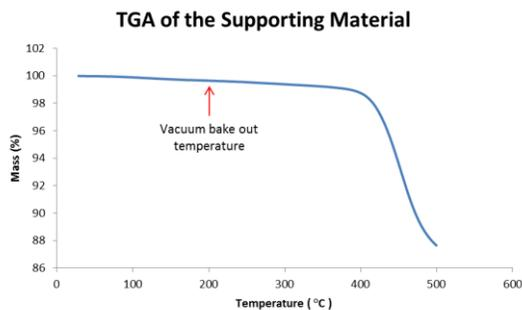
Fig. 2. Thermogravimetric analysis of the supporting material
